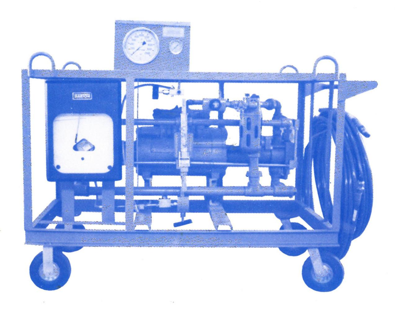
The B.O.P. Testing Unit consists of a MAC-28 two stage, pump, Barton pressure recorder, pressure gauges and discharge hose. The unit is mounted in an oil field type cage with casters. The unit is complete and ready to operate after hook-up to an air source and water source.
